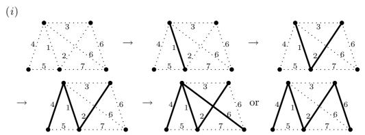
There are two solutions, because of the choice of "6"s at the last step. Note that "3" and "5", when they were the least weight unused edge, were not allowed, as each would make a circuit with already used edges.
