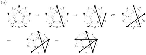
Although there was a choice of "6"s at the second step, both were eventually used anyway, so there was only one solution. Note that use of any of the "7"s would have made a circuit.
